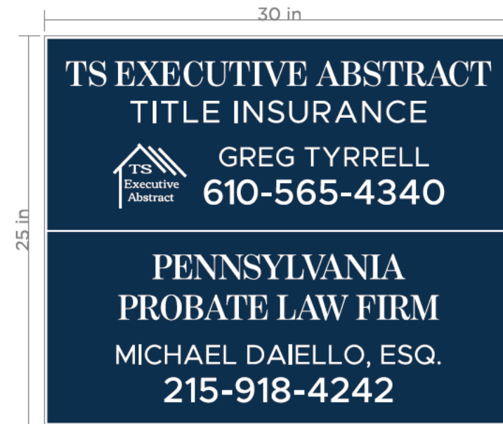
6 mm thick ACM with printed and gloss laminated vinyl graphics
