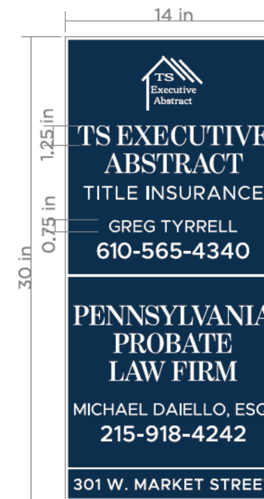
6 mm thick ACM with printed and gloss laminated vinyl graphics
