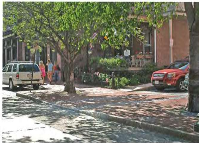
Crosswalk in driveway throat continuing the Sidewalk system
