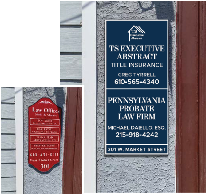
The existing building sign will be removed, and the new sign will be installed in its place with VHB tape and silicone.
