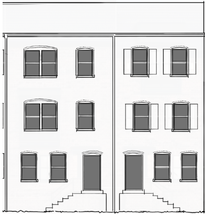
Illustration showing how openings on second and third floors should be aligned as customary in the historic buildings of the Borough.
