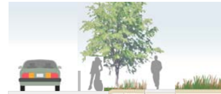
Proposed bike lane along S New St Lined with Flexible Bollards for Safety
